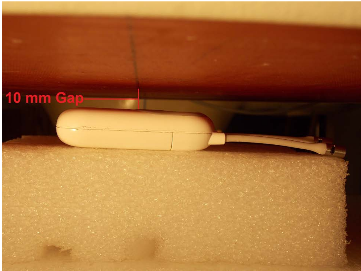
Test Position Face 10 mm Gap
