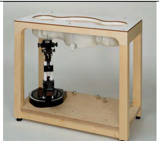
Fig. 8.7 Photo of SAM Twin Phantom
