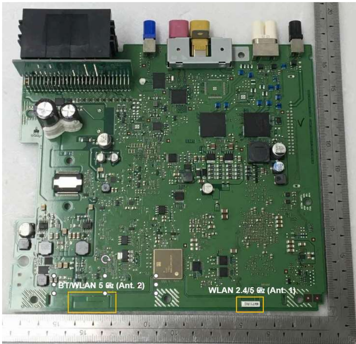
Figure F-1 WLAN Antenna Location
