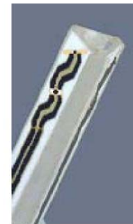
Figure 3.3 Probe Thick-Film Technique
