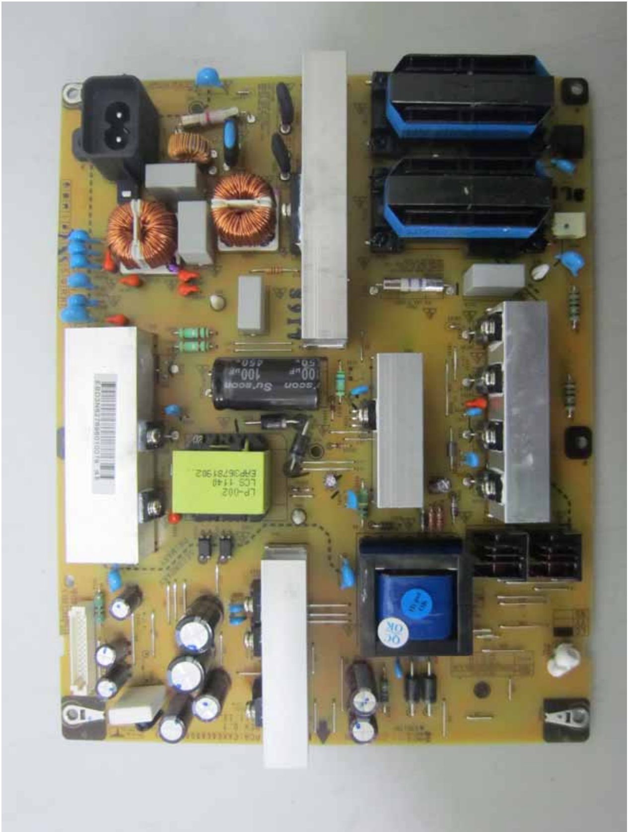
< Power Board Front >
