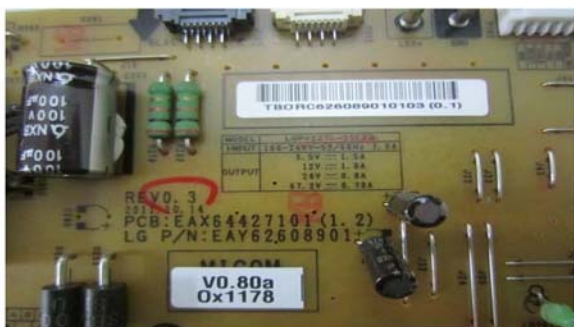
POWER BOARD LABEL(before)
