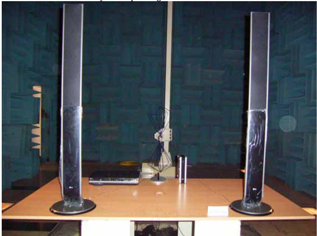
FRONT VIEW OF RADIATED MEASUREMENT
