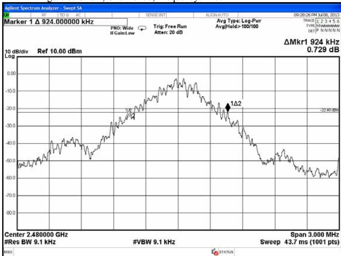
Figure 6: GFSK, Channel 78, Frequency: 2480MHz
