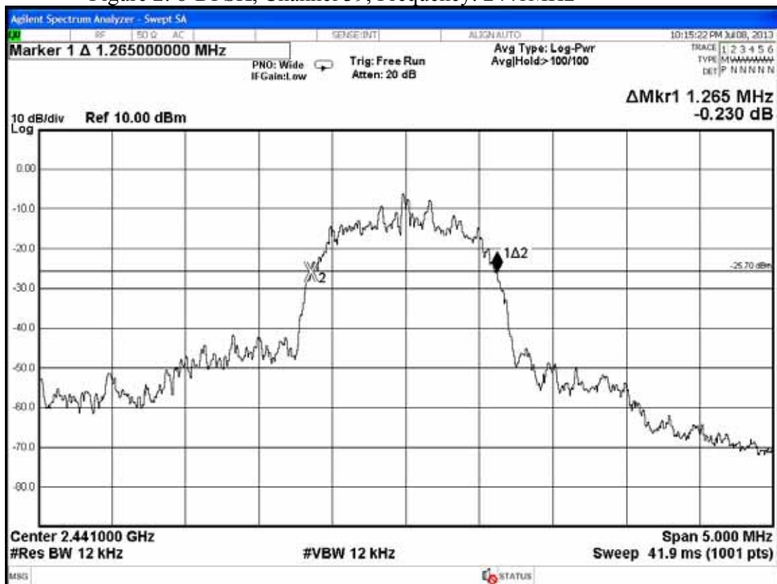
Figure 2: 8-DPSK, Channel 39, Frequency: 2441MHz
