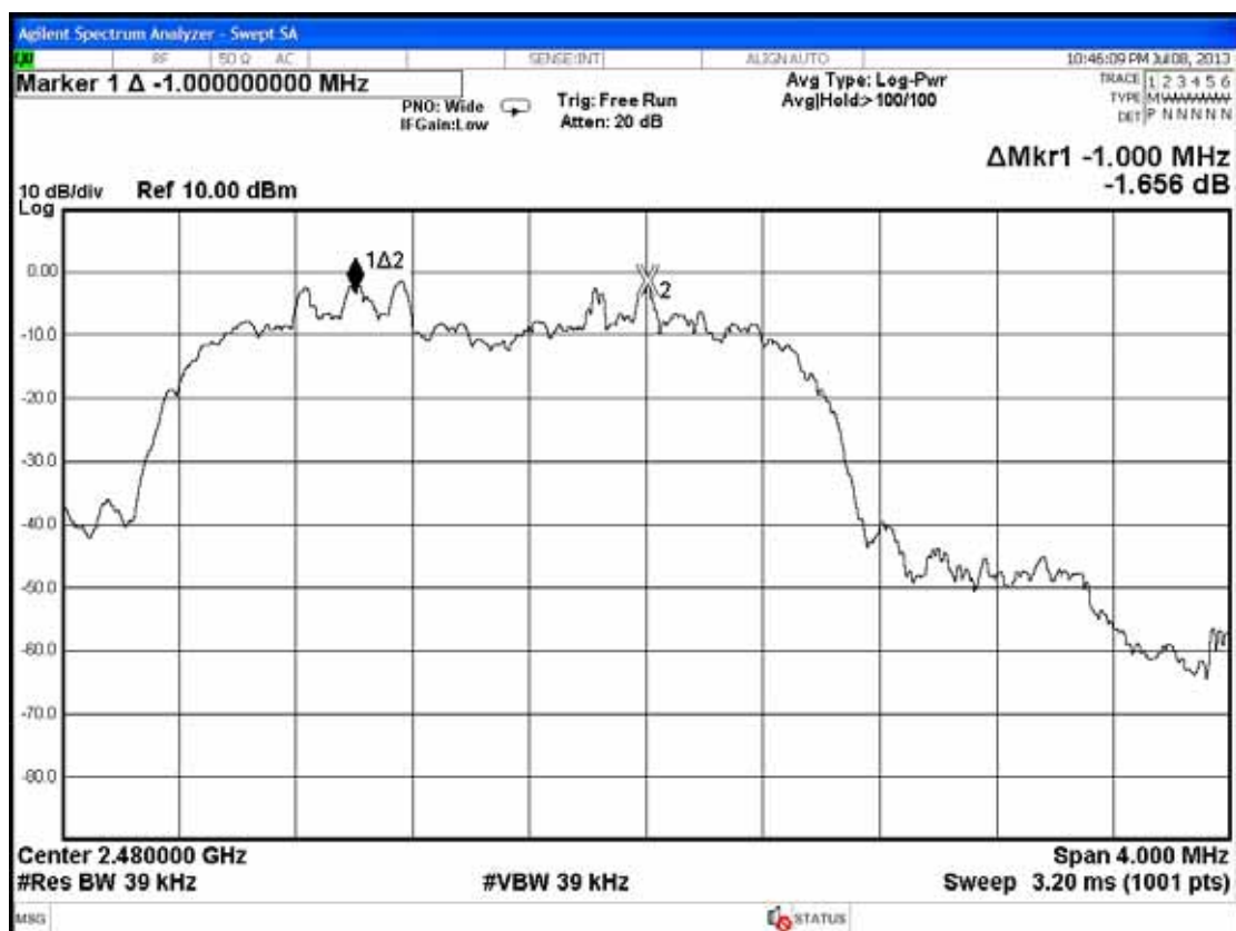
Figure 4: 8-DPSK, 2480MHz adjacent channel of carrier frequency separation
