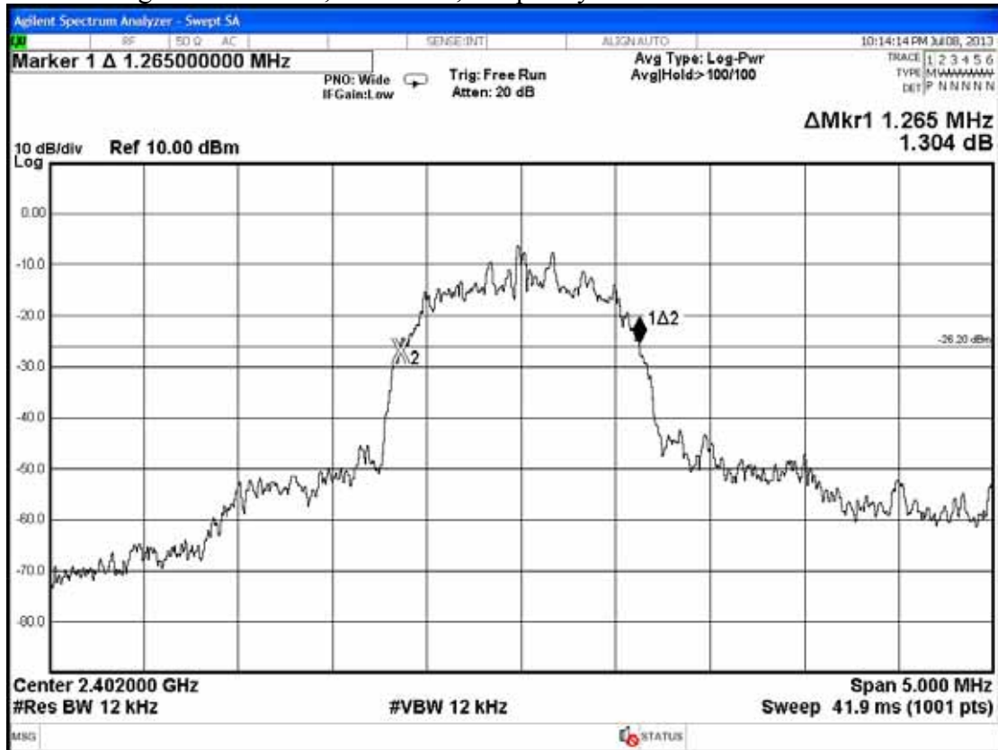
Figure 1: 8-DPSK, Channel 0, Frequency: 2402MHz
