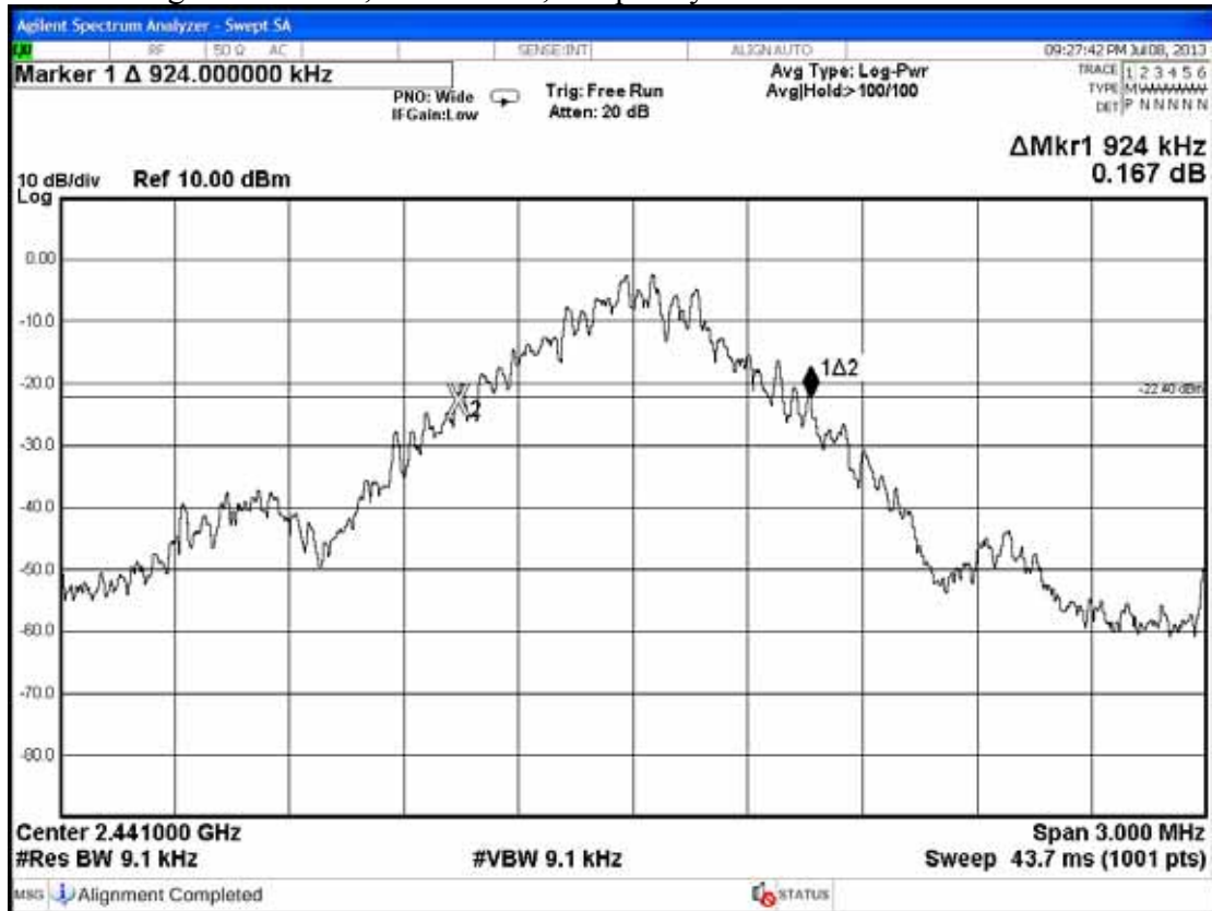
Figure 5: GFSK, Channel 39, Frequency: 2441MHz
