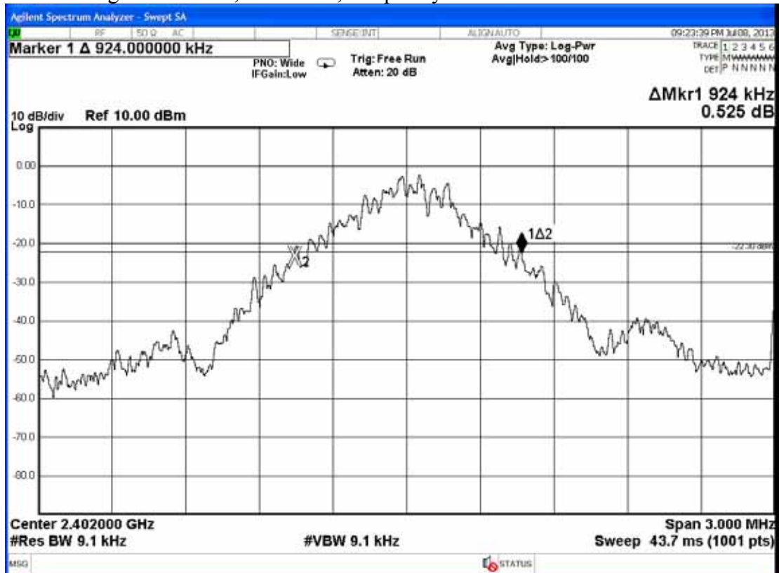
Figure 4: GFSK, Channel 0, Frequency: 2402MHz
