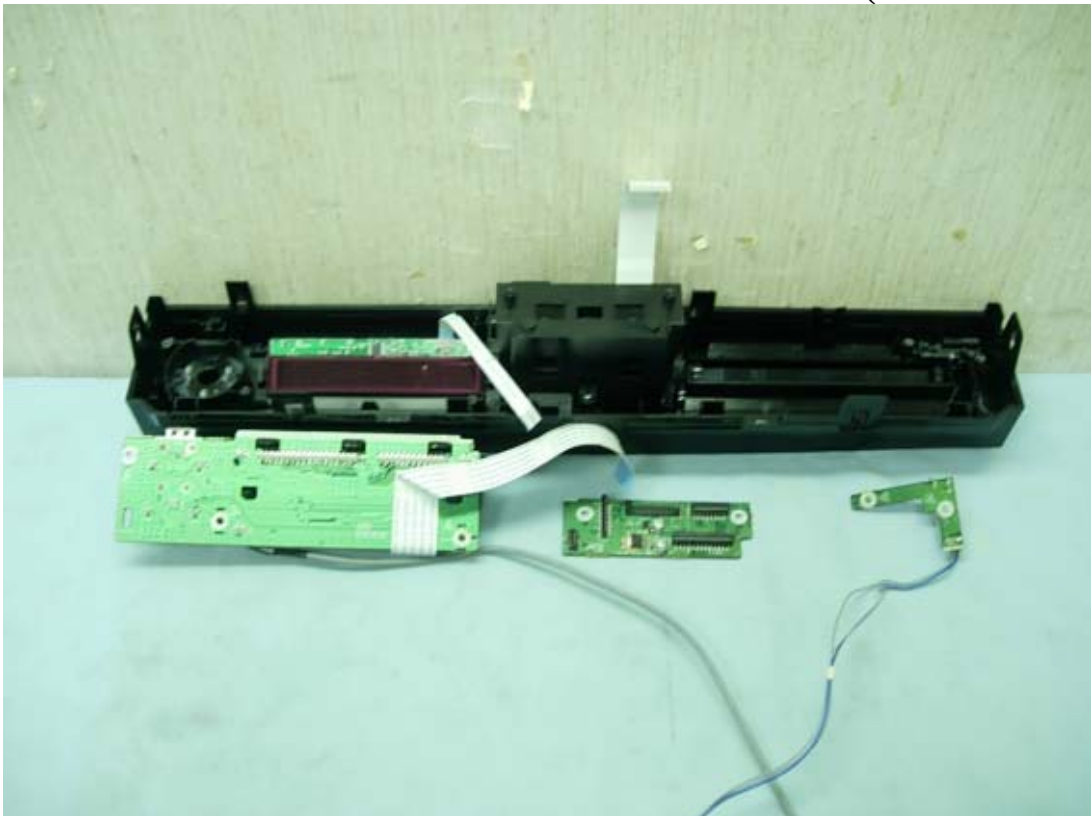
Figure 28 Internal View (Front Boards Removed)
