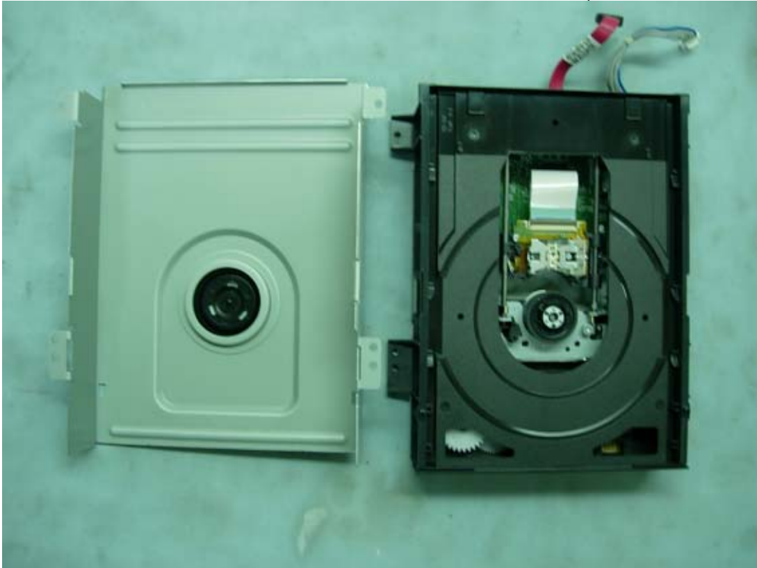
Figure 15 Internal View (DVD Driver, Front View)
