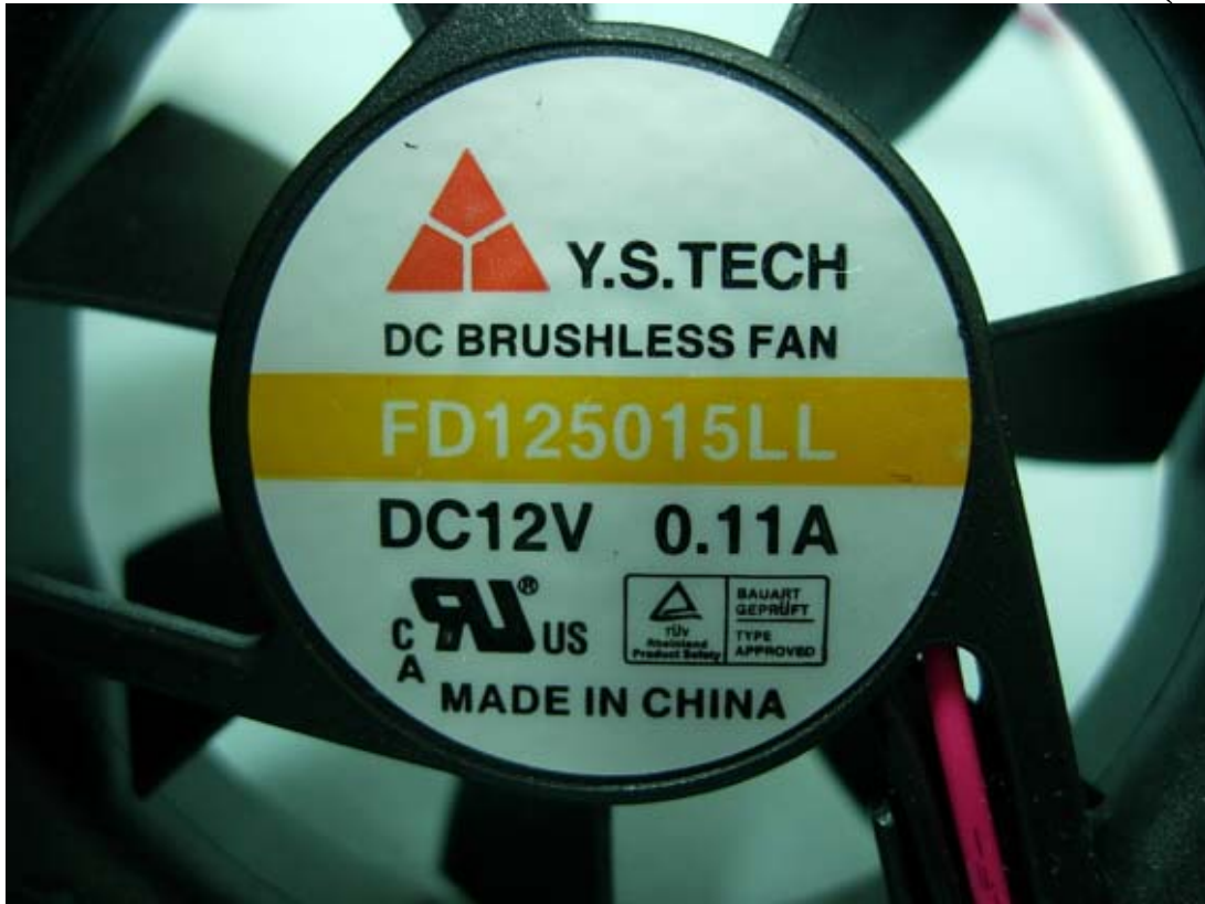
Figure 27 Internal View (Fan Label)
