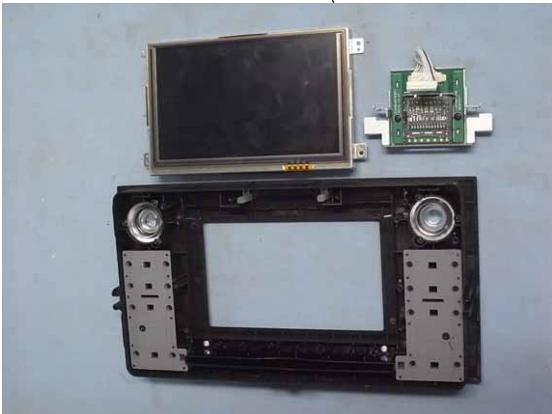
Figure 13 Internal View (Removed LCD Panel & Control Board)
