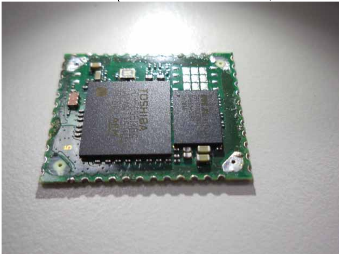
Figure 11 Internal View (Removed BT Module Metal Cover, BT Module/Front View)
