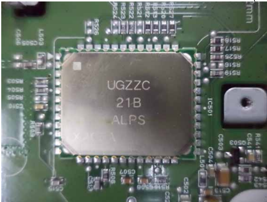
Figure 10 Internal View (BT Module)
