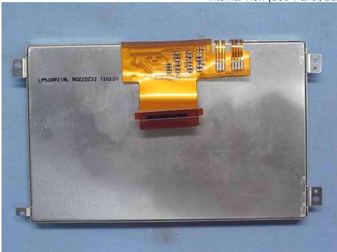
Figure 17 Internal View (LCD Panel, Back View)
