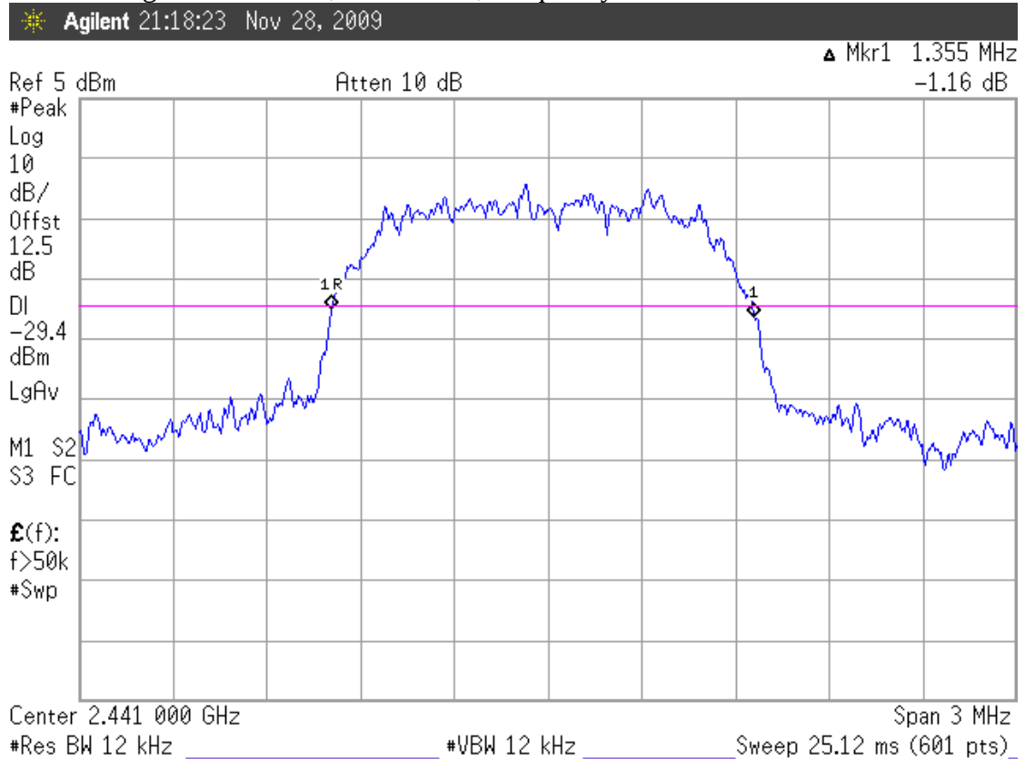
Figure 2: 8-DPSK, Channel 39, Frequency: 2441MHz
