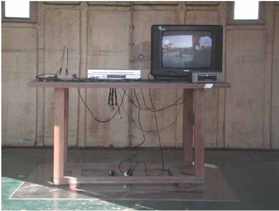
Photograph of Test Set-up ( Power line radiated emissions)
