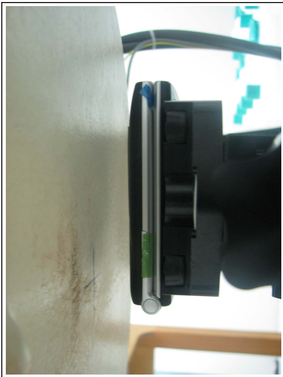
Figure 6 Body SAR Test Setup – w/o Holster
