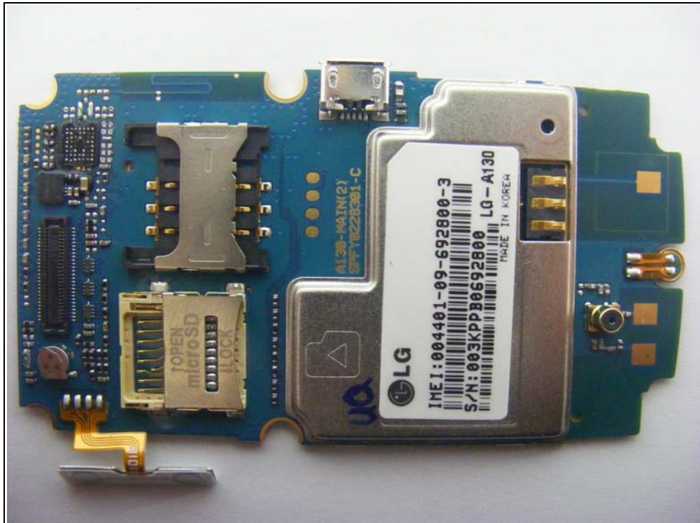
Top view of Main PCB Removing Shield
