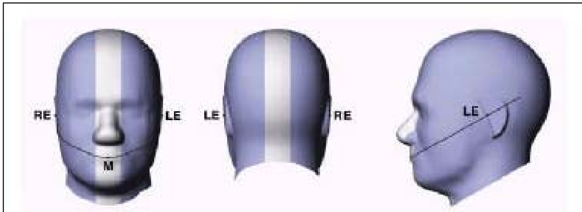
Figure 6.1 Front, back and side view of SAM Twin Phantom
