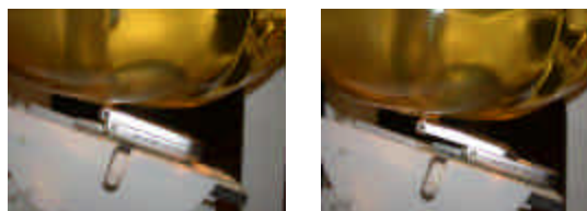
Figure A.2 Right Head SAR Test Setup -- Ear / 15° Tilt Position --
