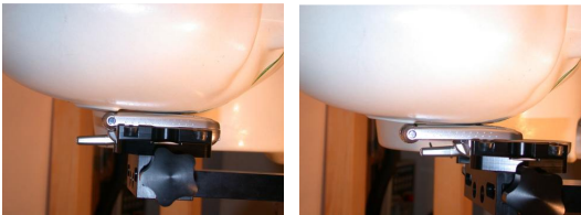
Figure 14.5 Right Head SAR Test Setup -- Cheek / Touch Position --
