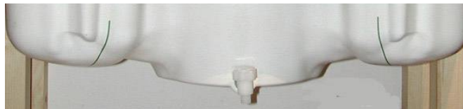
Figure 7.2 SAM Twin Phantom shell
