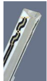
Figure 3.2 Probe Thick-Film Technique
