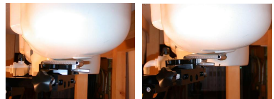
Figure 14.7 Left Head SAR Test Setup -- Cheek / Touch Position --
