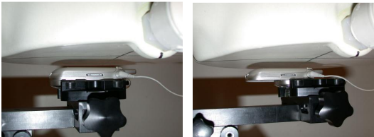
Figure 14.10 Body SAR Test Setup -- w/o Belt-clip --
