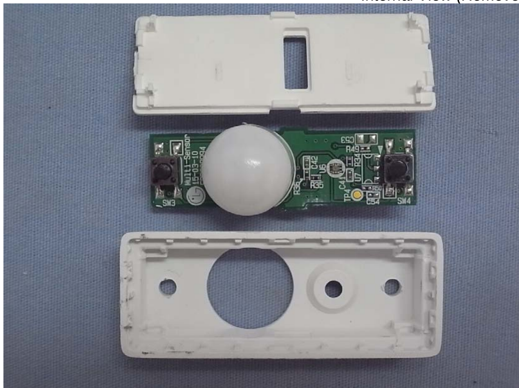
Sensor Figure 9 Internal View (Removed Covers)
