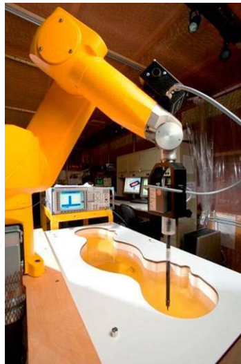
Figure 3-2 DASY4 SAR Measurement System
