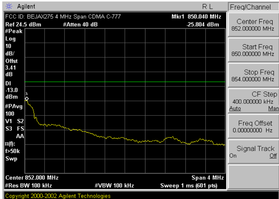
Plot 7-25. 4MHz Span Plot (Cellular CDMA Mode – Ch. 777)
