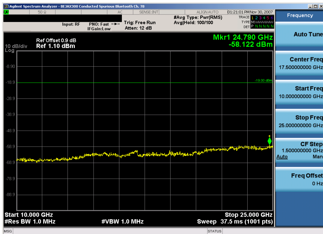
Plot 6-17. Conducted Spurious Plot (Bluetooth – Ch. 78)
