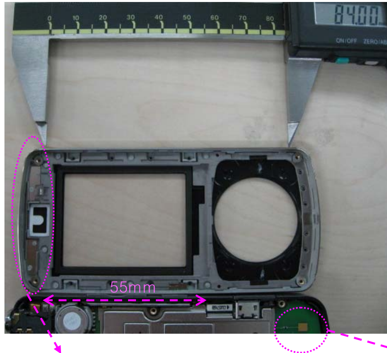
FM Transmitter Antenna
