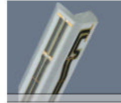
Figure 5-1 E-field Free-space Probe
