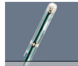
Figure 5-2 H-Field Free-space Probe
