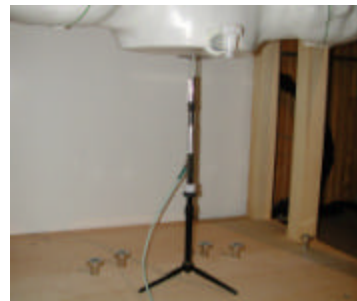
Figure 12.1 Dipole Validation Test Setup
