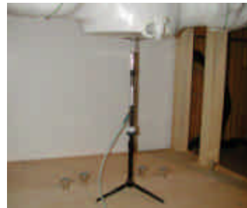
Figure 12.1 Dipole Validation Test Setup
