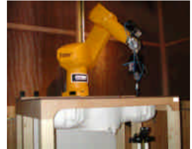
Figure 6.1 DASY4 Test System
