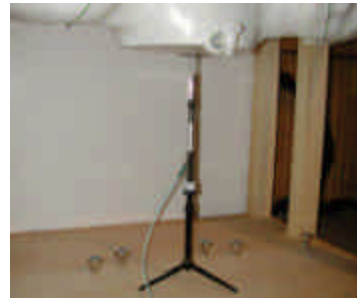
Figure 12.1 Dipole Validation Test Setup
