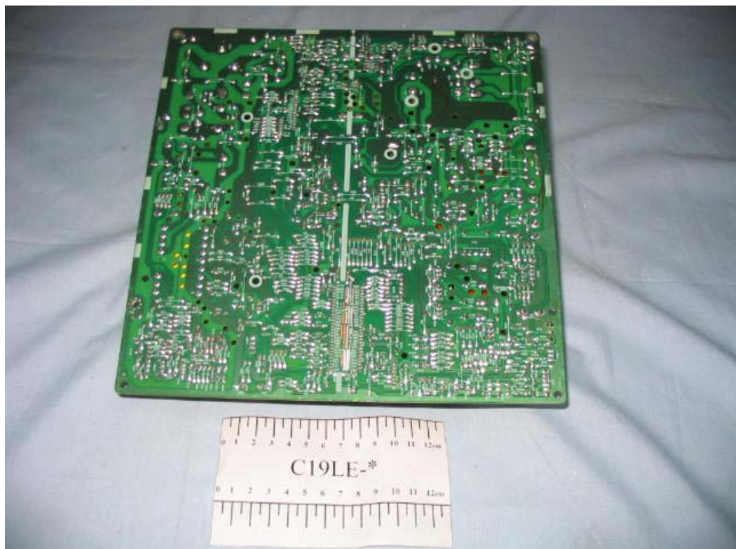
FIGURE 6 COLOR MONITOR (M/N:C19LE-*) MAIN BOARD (SOLDERED SIDE)
