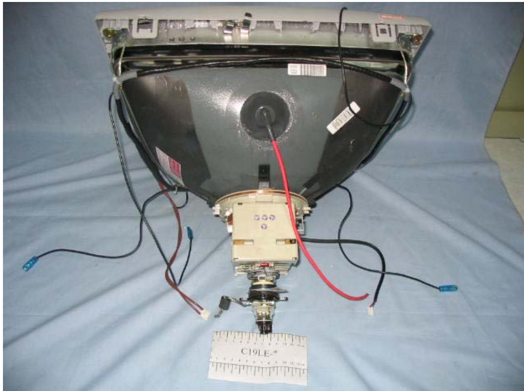
FIGURE 3 COLOR MONITOR (M/N:C19LE-*) CRT TUBE
