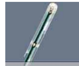
Figure 5-2 H-Field Free-space Probe
