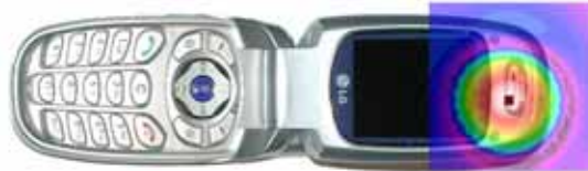
Figure A T-coil Location
