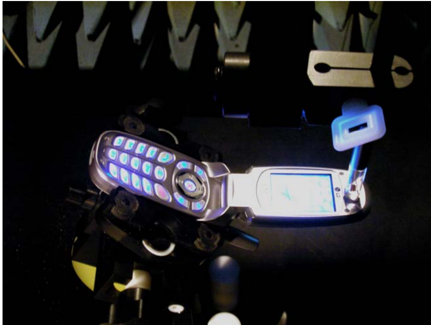
Figure 12-1 Test Setup for Wireless Device
