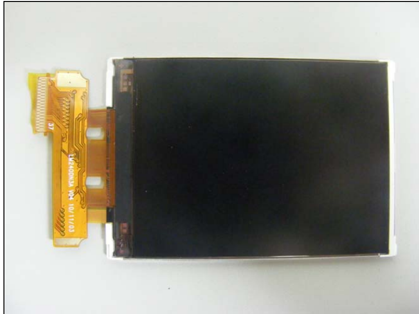
Bottom view of LCD module
