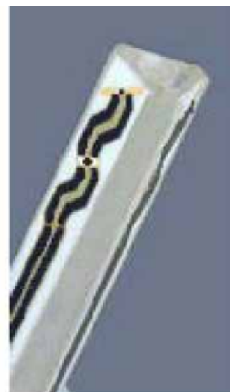
Figure 3.3 Probe Thick-Film Technique
