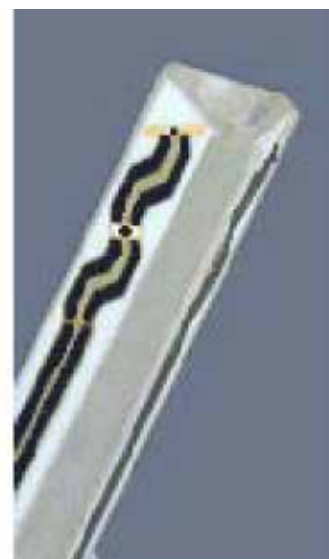
Figure 3.3 Probe Thick-Film Technique
