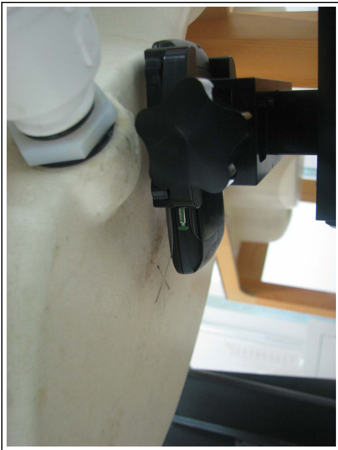
Figure 5 Mouth SAR Test Setup – w/o Holster
