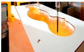
Figure 6-2 SAM Phantom with Simulating Tissue
