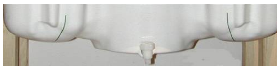
Figure 7-2 SAM Twin Phantom Shell
