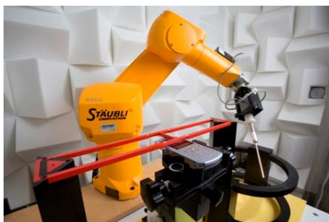
Figure 5-5 SPEAG Robotic System
