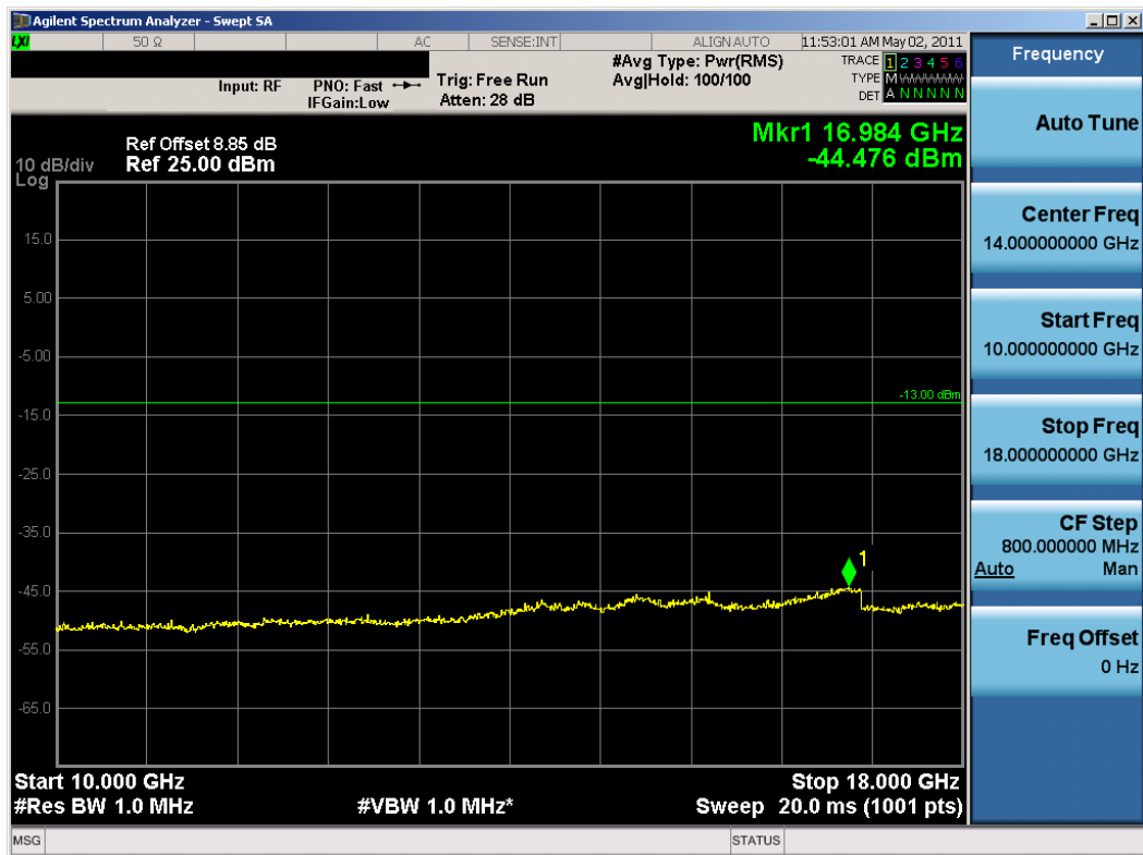
Plot 7-28. Conducted Spurious Plot (AWS WCDMA Mode – Ch. 1412)
