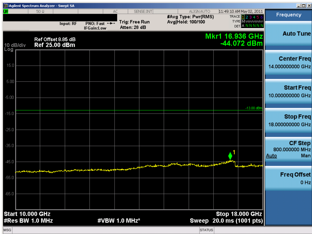
Plot 7-24. Conducted Spurious Plot (AWS WCDMA Mode – Ch. 1312)
