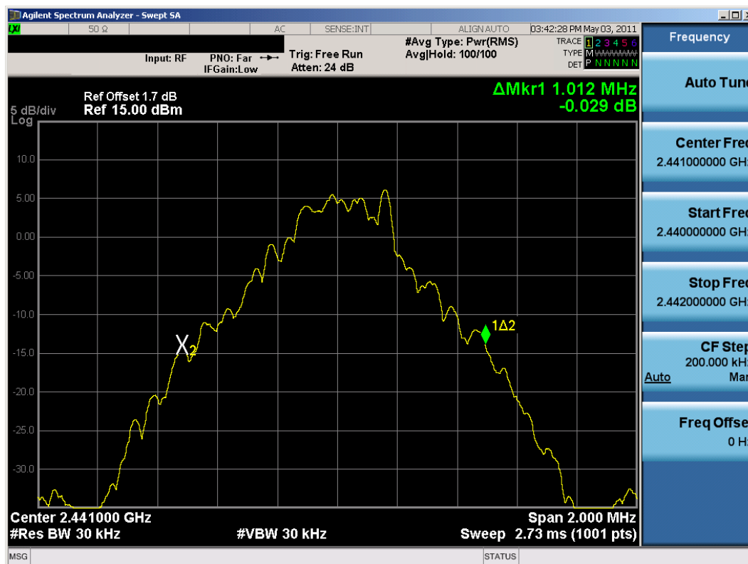
Plot 6-2. 20dB Bandwidth Plot (Bluetooth, 1Mbps - Ch. 39)
