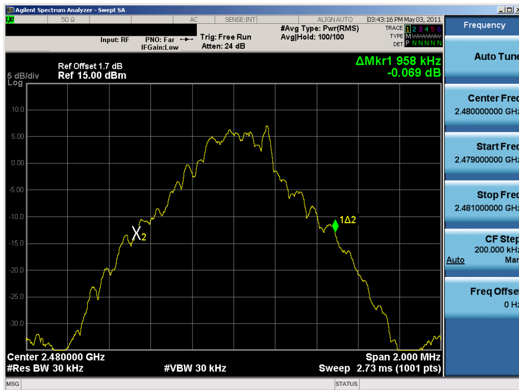
Plot 6-3. 20dB Bandwidth Plot (Bluetooth, 1Mbps – Ch. 78)
