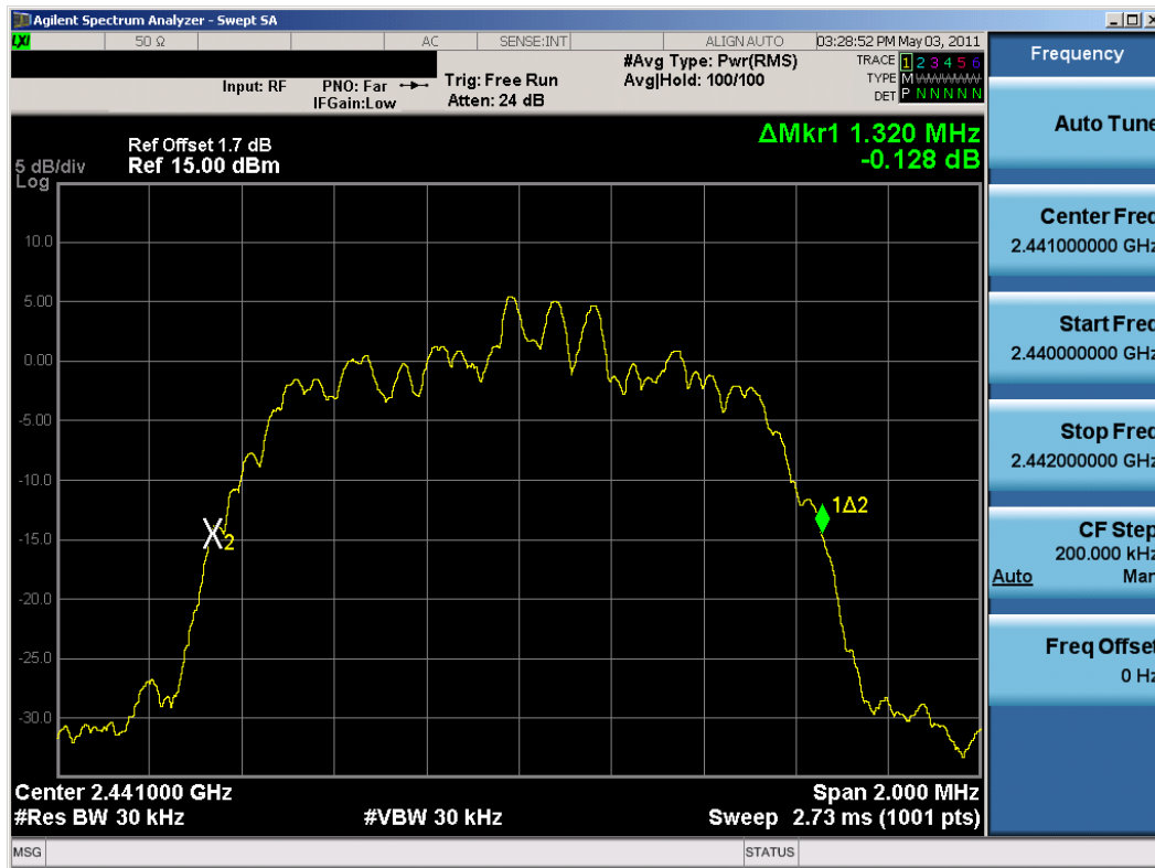
Plot 6-5. 20dB Bandwidth Plot (Bluetooth, 2Mbps – Ch. 39)
