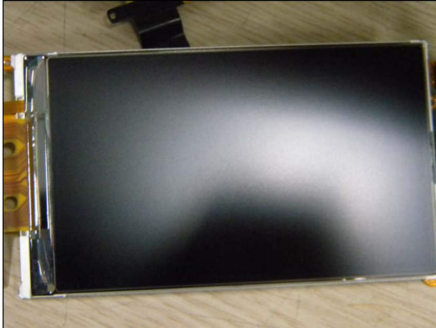
Bottom view of LCD Panel
