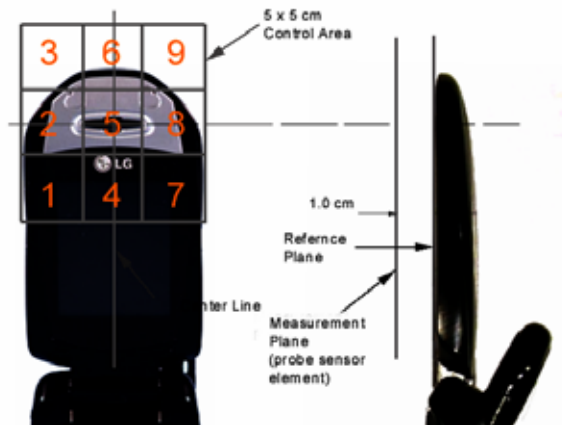
Figure 13 E/H-Field Emissions Test Setup Diagram
