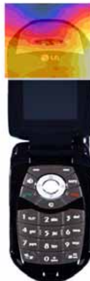
Figure 28 Sample H-field Scan Overlay
