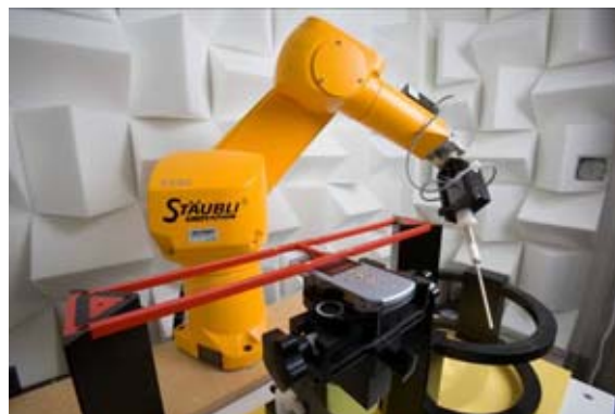
Figure 3-1 HAC Assessment System
