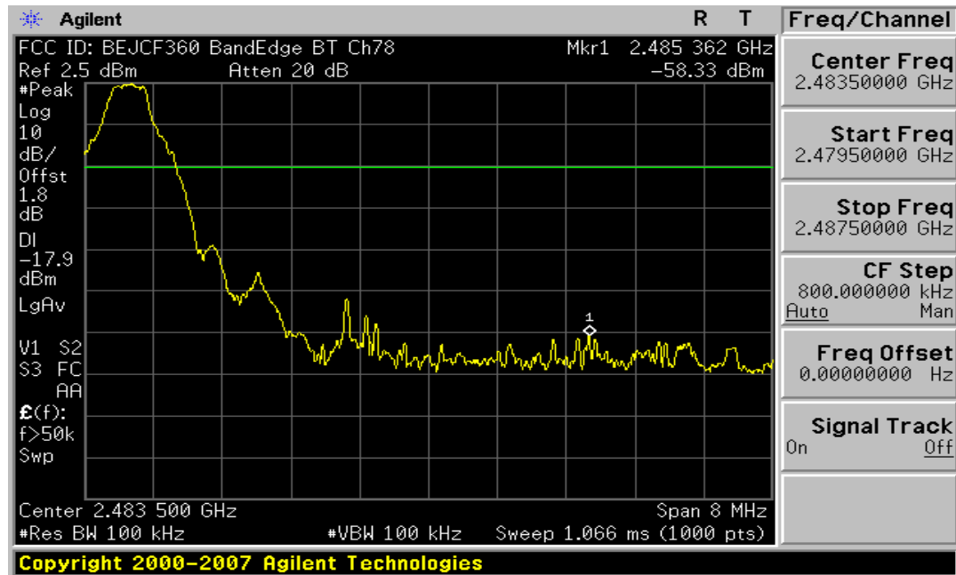
Plot 6-5. Band Edge Plot (Bluetooth – Ch. 78)
