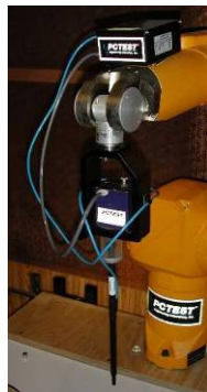
Figure 5-7 SPEAG Robotic System
