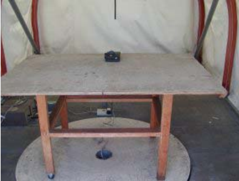
Base Conducted Emission Setup Photograph - Front View
