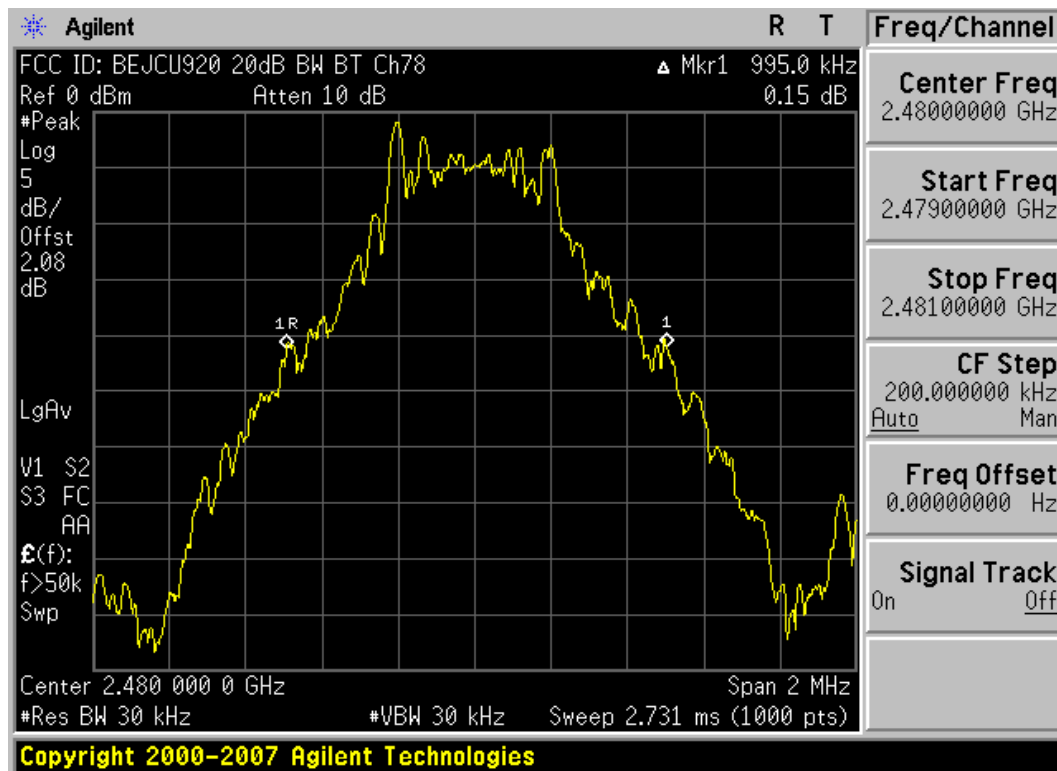
Plot 6-3. 20dB Bandwidth Plot (Bluetooth – Ch. 78)
