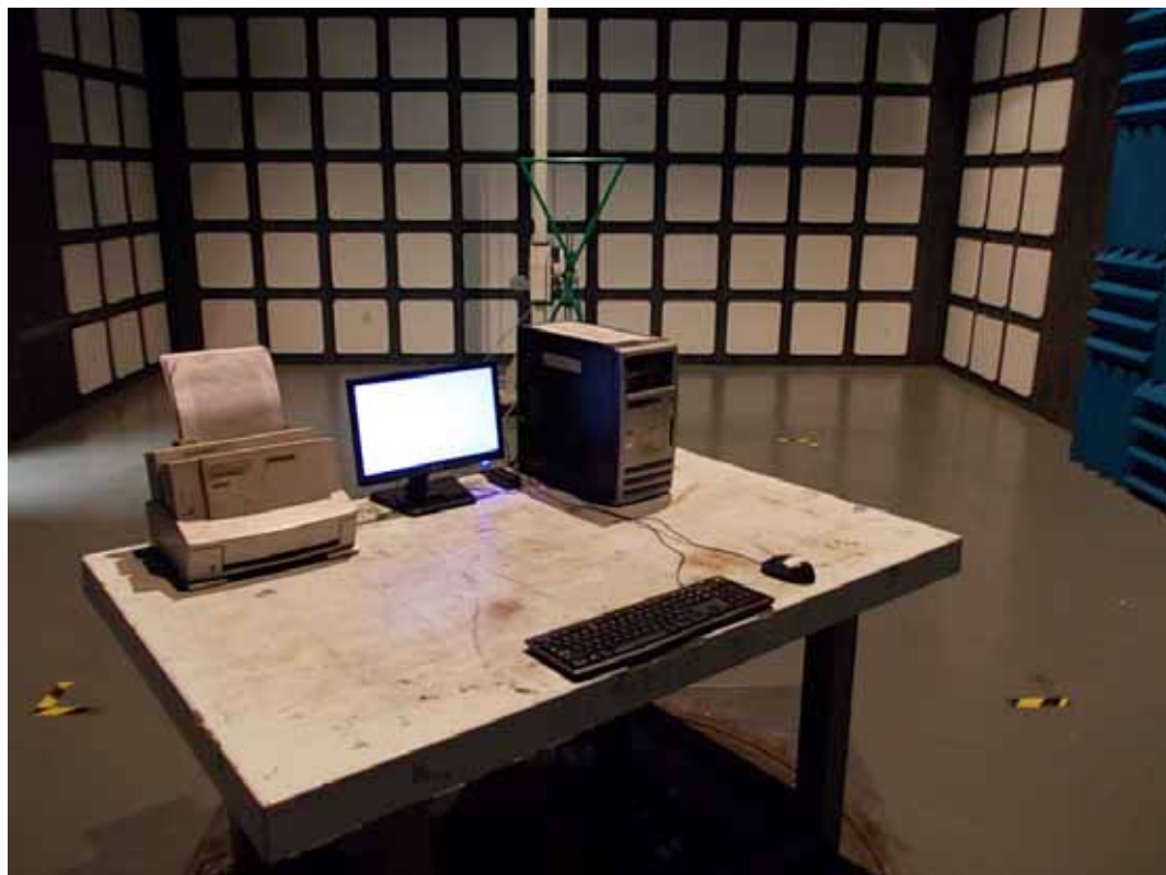
SETUP WITH MAXIMUM DETECTED EMISSION AT VERTICAL POLARIZATION (TEST MODE: D-SUB 1366*768@60Hz ADAPTER #1)
