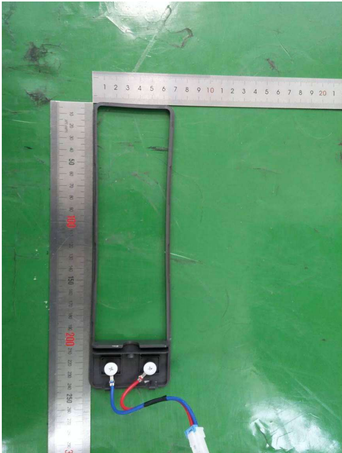
<Pillar Heater Section-1>
