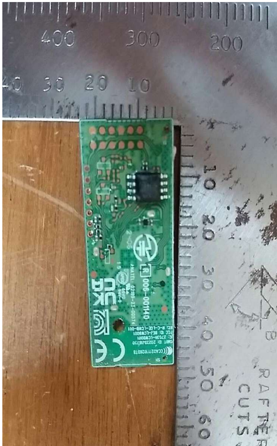
Alternated New Item_< Wi-Fi module Section -2>
