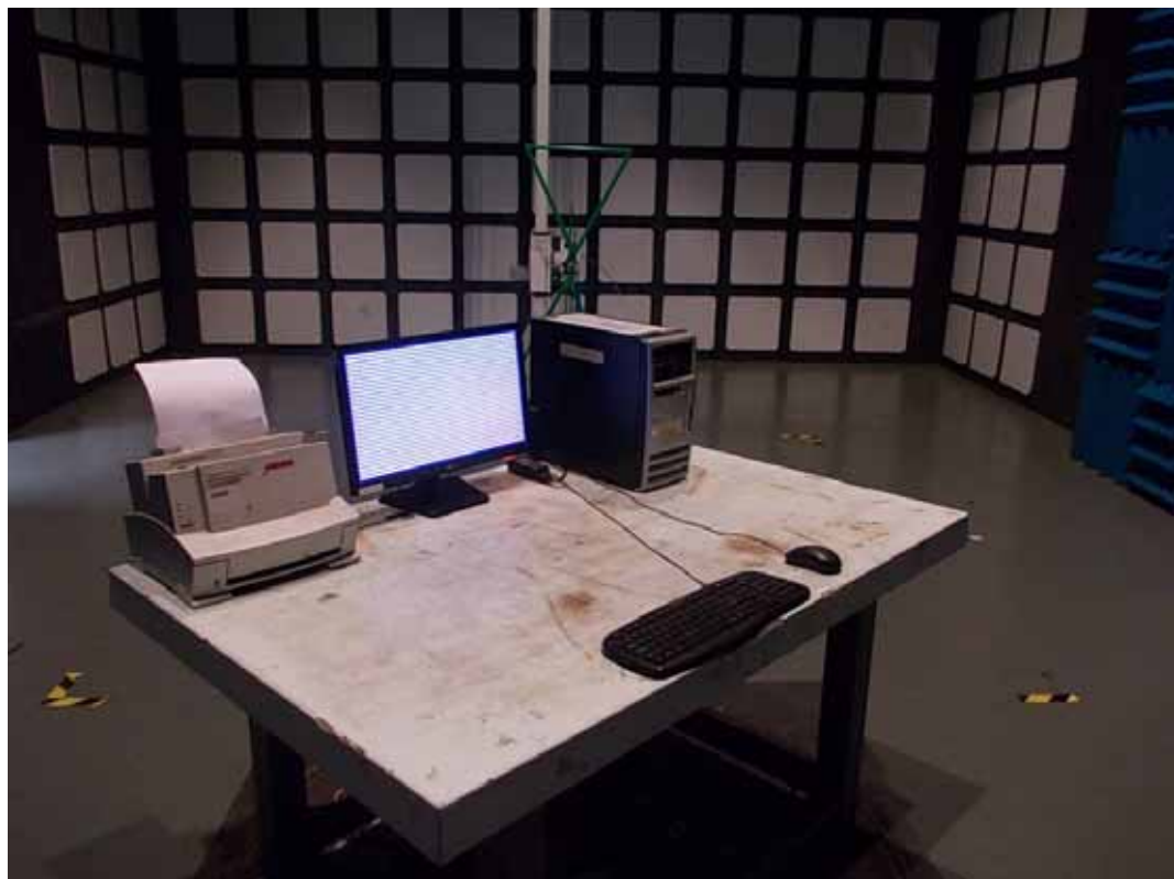
SETUP WITH MAXIMUM DETECTED EMISSION AT VERTICAL POLARIZATION (TEST MODE: DVI 1920*1080@60Hz Adapter #1, Panel #1)
