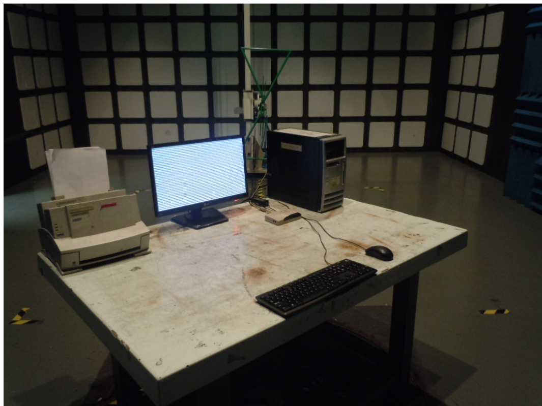
SETUP WITH MAXIMUM DETECTED EMISSION AT VERTICAL POLARIZATION (TEST MODE: DVI 1920*1080@60Hz ADAPTER #2, PANEL #2)
